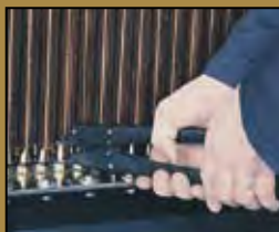
Hand tool lifts tube from seal.
