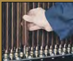
Tube is removed from header plate.
