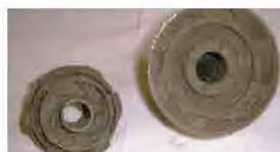
ESP pulled from well due to inefficiency from scale deposits
